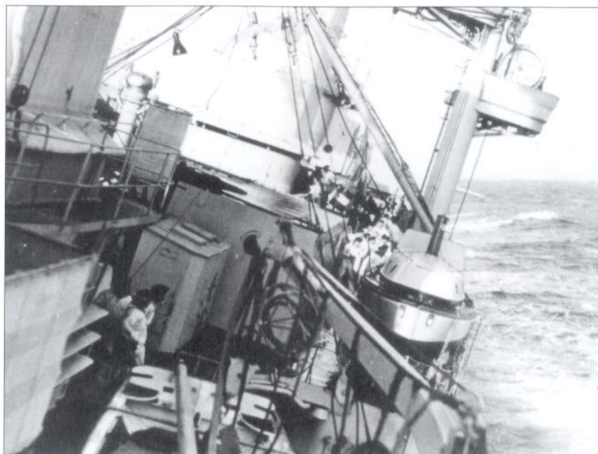
The K-class cruisers had a tendency to roll even in a moderate swell, as shown here. This view, looking astern from the bridge area, shows the ship's boats nearest the camera, a pinnacle and the derrick with the searchlight platforms.
