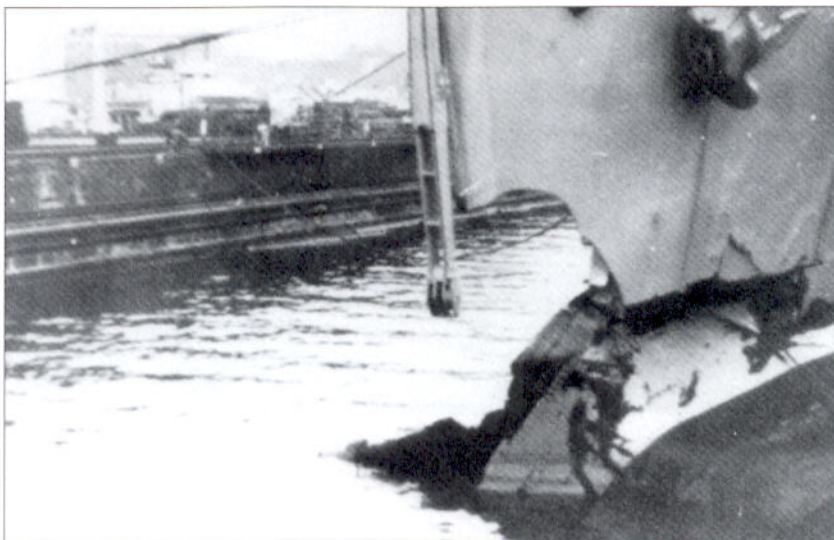
Nürnberg's bow, showing the damage she suffered in the torpedo attack on 1939. Fortunately, her internal bulkheads held and she was able to return safely to harbour. Note that her heraldic shield is still in place, suggesting it was some little time after the outbreak of war before these insignia were removed from all ships.
